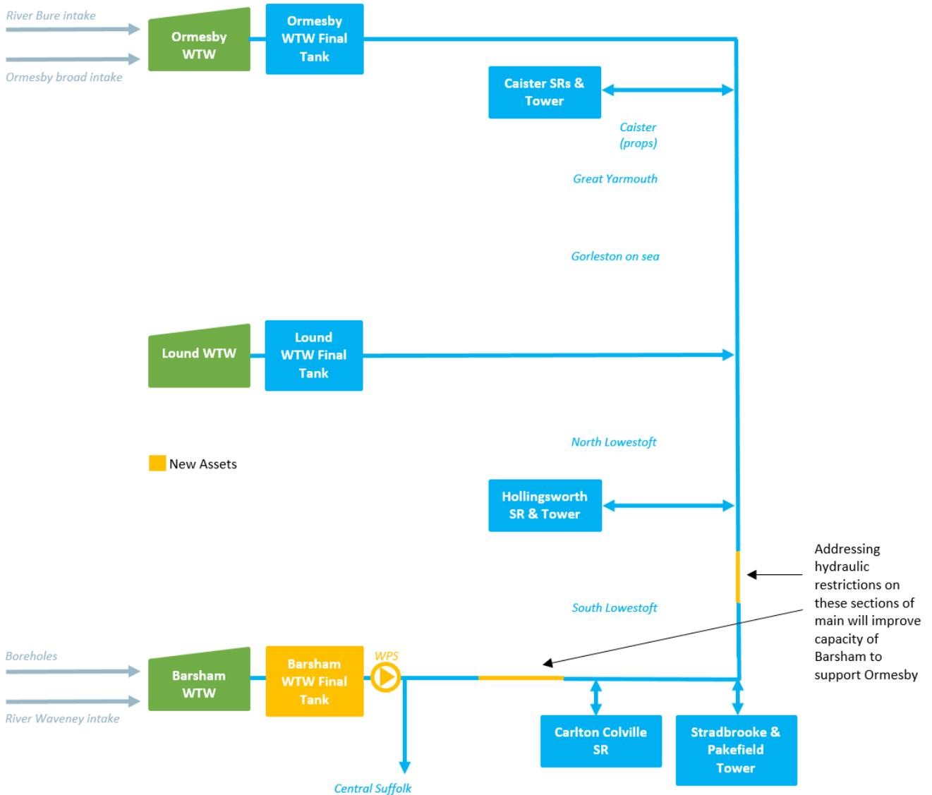
**Figure 2: North Suffolk zone schematic highlighting proposed solution**
