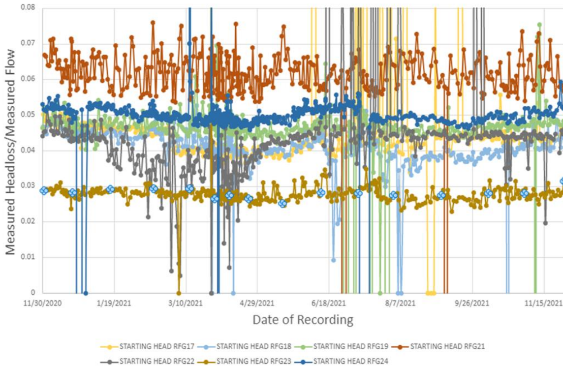
FIGURE 17: HANNINGFIELD WTW – NORMALISED FILTER HEADLOSS AFTER BACKWASH CYCLE
