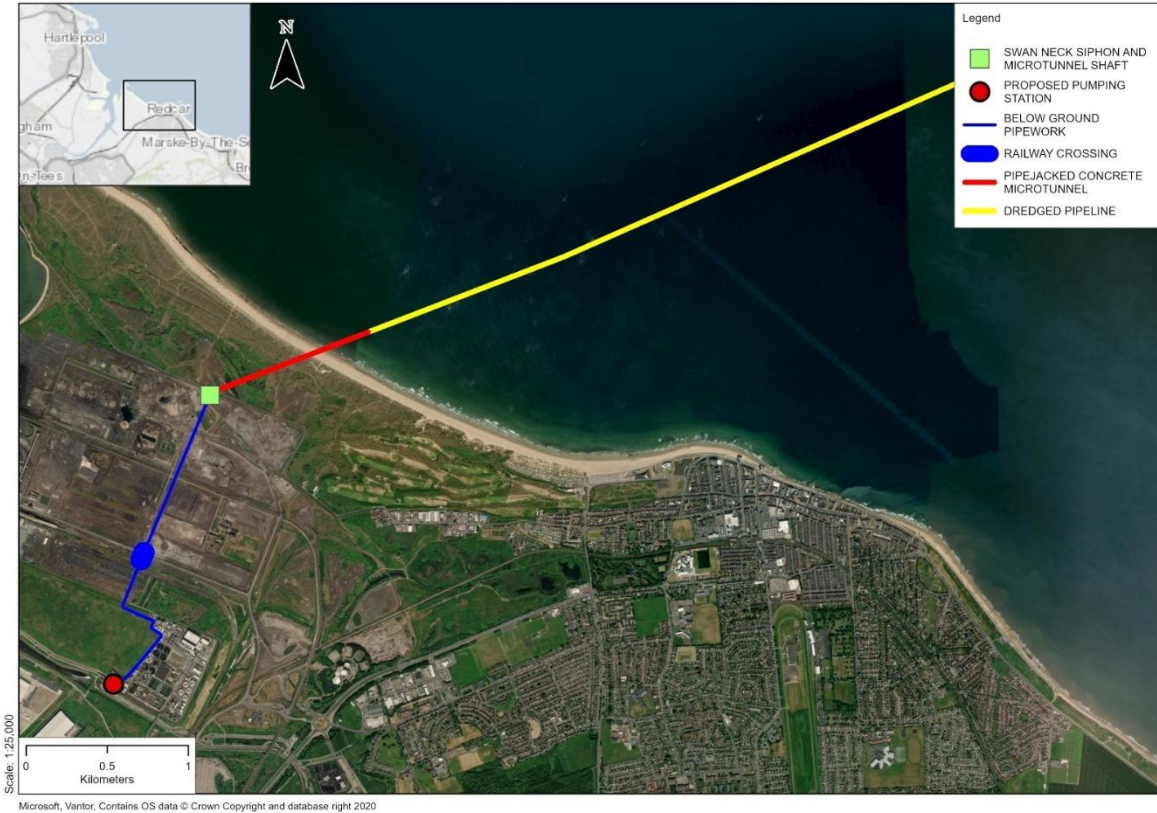
FIGURE 5 - LOCATION PLAN – PUMPING STATION, PIPELINE AND OUTFALL
