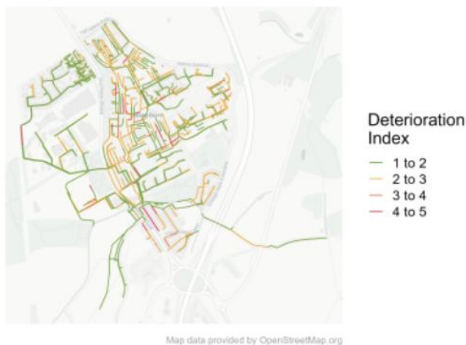
Binned Sewer Condition Grade Predictions Bowburn
