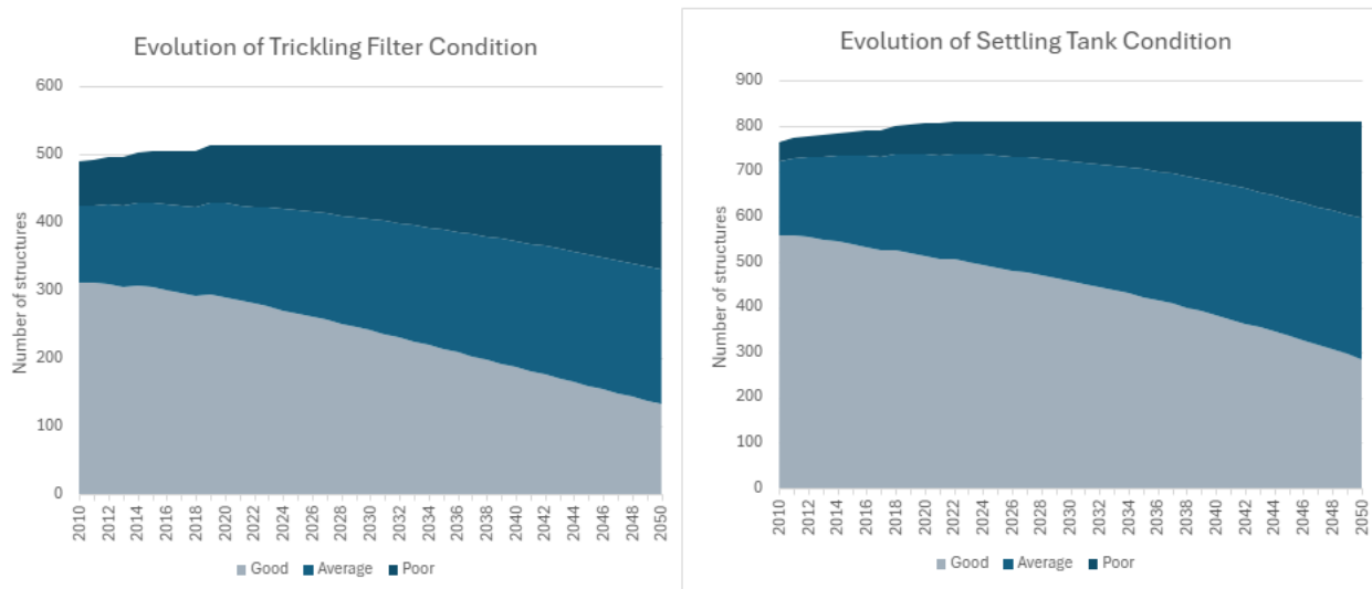
FIGURE 14 - EVOLUTION OF CONDITION FOR SETTLEMENT TANKS AND TRICKLING FILTERS
